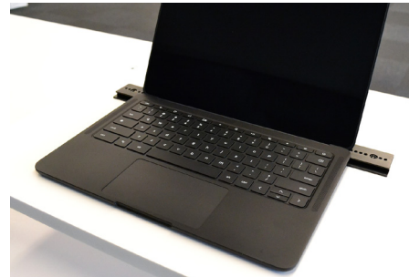
20 Center the laptop on the rail to determine the position of the locks.
