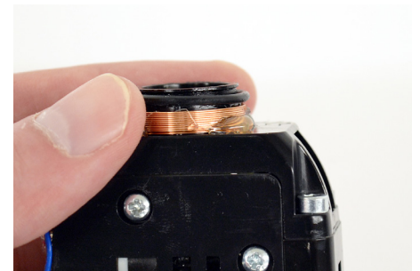
16 Place the smaller circular gasket in the groove near the IR port.
